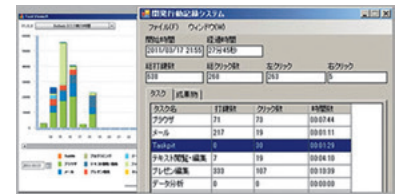
Fig. 2 TaskPit: A software development task measurement system
