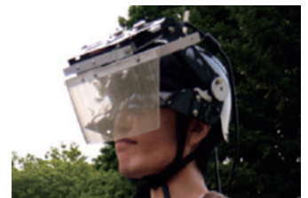
Fig. 4 Super wide field of view optical see-through HMD
