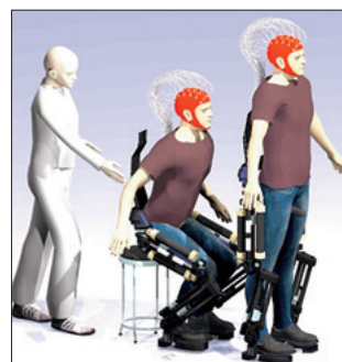
Fig. 7 Adaptive shared control for BMI exoskeleton robots
