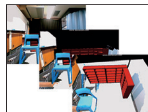
Fig. 7 An AR furniture arrangement system that automatically shifts to the optimal viewpoint
