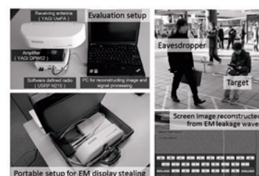
Fig. 1 Remote Visualization of Screen Images Using EM Emanation
