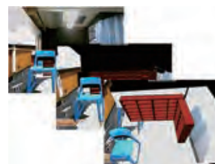
Fig. 7 An AR furniture arrangement system that automatically shifts to the optimal viewpoint
