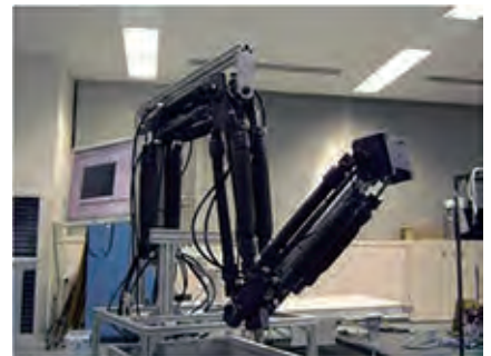
7-DOF manipulator controlled by pneumatic artificial muscles (Mathematical Informatics Lab)
